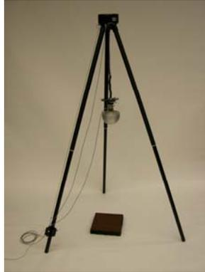
Figure 3 - Tripod with Head form hanging & reference pad
